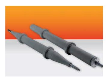
Furnace rollers made from Kanthal APMT, an iron-chromium-aluminium (FeCrAl) alloy, for heat treatment furnaces with operating temperatures up to 1250°C (2280°F). Kanthal furnace rollers are available in outside diameters from 26 to 260 mm (1 to 10 in.), according to customer design.
