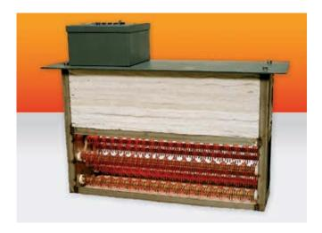
With Kanthal air heating cassettes it is possible to heat air or gases up to 800°C (1470°F) and maintain a uniform temperature throughout the oven, furnace or process equipment. The air heating cassettes can be produced to fit most existing or new furnace designs. Installation is very simple in most cases.
